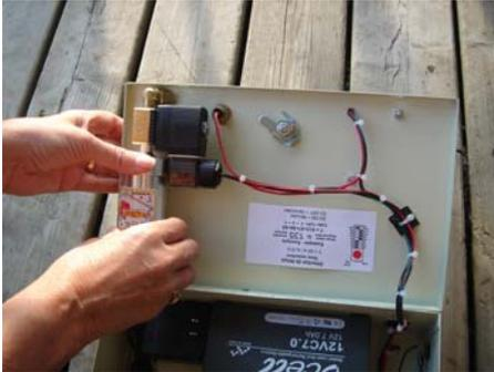
To refill, open the door panel with the round key, unscrew anti-clockwise, by the bottom of the canister, replace the canister and screw clockwise. Do not use an excessive force. Close the door.
