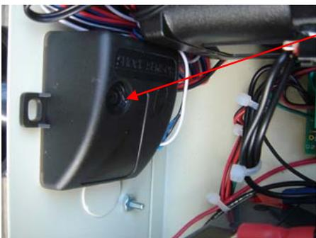
The shock sensor detector is adjustable with the small screw; when turned on the left, it is less sensitive and if turned on the right, it is more sensitive. Preferably, keep the manufactory settings as they are, otherwise the system can be easily activated and spread the Cayenne pepper.
