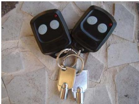
**To arm the system:** wait 120 seconds after the system is on. From a maximum distance of 75 feet's, press and immediately release the remote's left button (with the lock), the alarm will sound and the red LED will start blinking. At that time, you have 30 seconds to leave the area. After the first 10 seconds, the alarm will sound 4 times, at that point, there is 20 seconds remaining to leave the area (manufactory setting).
