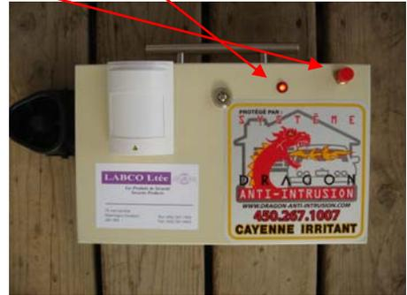
Place the portable DRAGON ANTI INTRUSION system upright, the moving detector faced towards the protected area, from 3 to 7 feet's height, depending on the distance required; for example: 3 feet height = about 10 feet distance, 7 feet height = about 35 feet distance. Arm and leave the area immediately.
