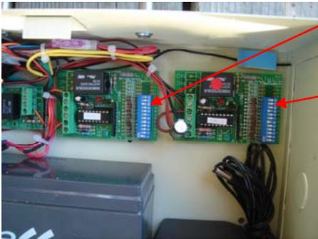
The left circuit is for the pepper spray delay. The right circuit is for the outing time delay.
