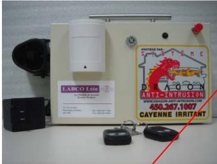
To put the system on, open the panel door with the round key. Pull the switch towards and close the panel. The LED will turn on red. Take the DRAGON red cap off.
